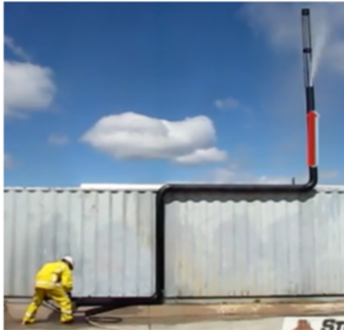
fig. 7 self propelled cleaning head
